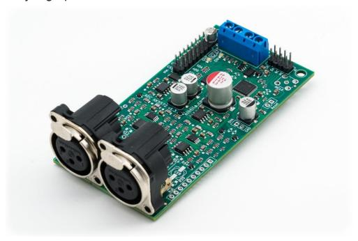
ADC AK5572 is a very high performance audio ADconverter suitable for sound recording applications or high end audio setups. Alternatively, using this ADC in a DIY audio analyser system one can build a very capable setup when paired with a suitable PC software.
