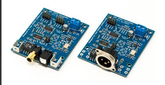
SPDIF TX is an I2S to S/PDIF digital audio converter. It takes in I2S serial audio data in either conventional stereo format or specific dual mono format used in nihtila.com ADC AK5572 AD-converter.
