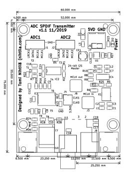
Sample rate selection with jumper links J4. Sample rate fs depends on Master Clock; MCLK is integer multiple of fs. Values are given for 24.576 MHz MCLK.
