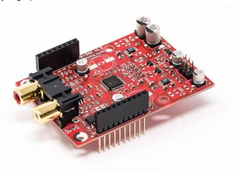
W-DAC 4493 is a very high performance audio DAconverter suitable for the most demanding DIY DAC setups. Despite compact size and humble looks, performance figures are impressive reaching 121 dBA dynamic range, -115 dB THD+N, and -121 dB THD.
