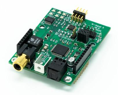
W-Input S is a software/I2C controlled version of W-Input, a compact digital audio input board. W-Input S supports up to 8 S/PDIF inputs with up to 192 kHz / 24-bit audio. In addition, another input offers a direct I2S passthrough supporting any sample rate. This allows for using external I2S source, such as USB to I2S module.
